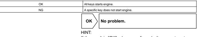
If the result is "OK", please confirm whether or not customers have ever inserted the unregistered key or the immobiliser key (with transponder chip) of other vehicle in the ignition key cylinder, and find out the cause of detecting DTC.
